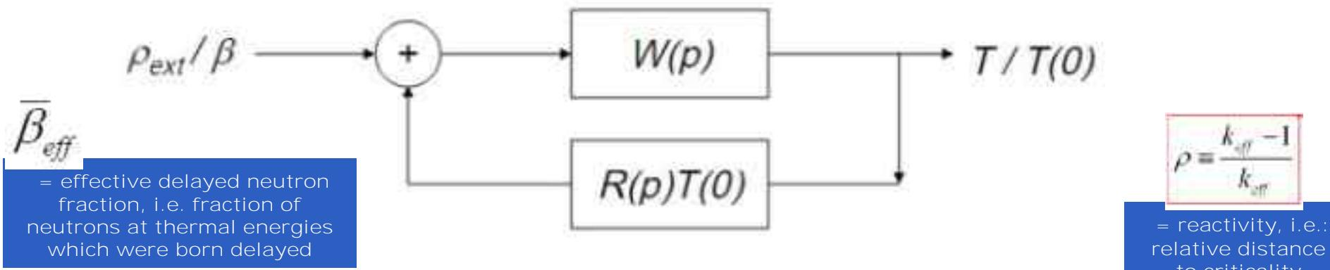
Transfer function of the reactor with feedback
