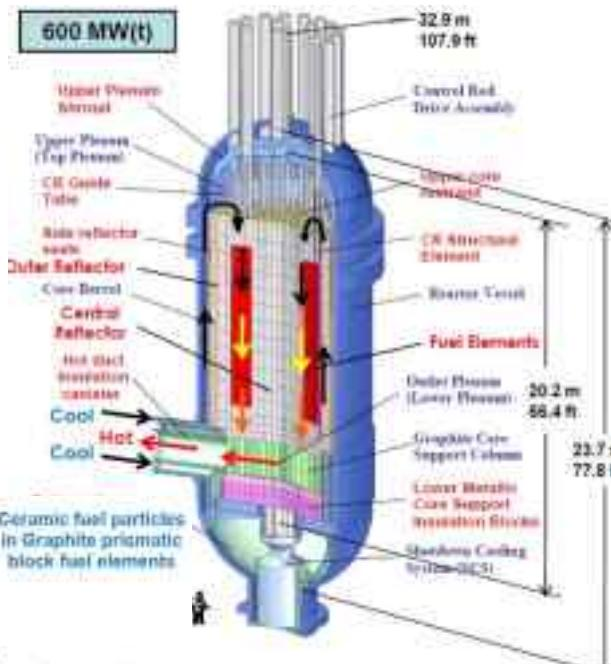
The tristructural-isotropic (TRISO) coated particles are embedded in cylindrical compacts of graphite matrix material with a diameter of slightly more than 1 cm, and the compacts are loaded into graphite fuel blocks.
