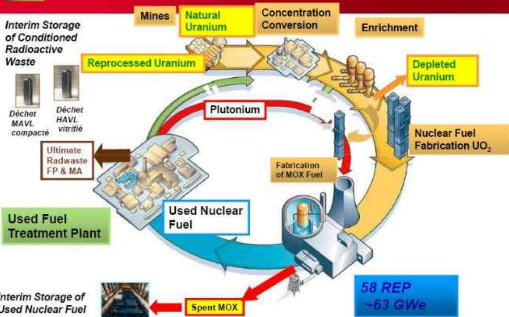
Fuel removed from a reactor, after it has reached the end of its useful life, can be reprocessed to produce new fuel
