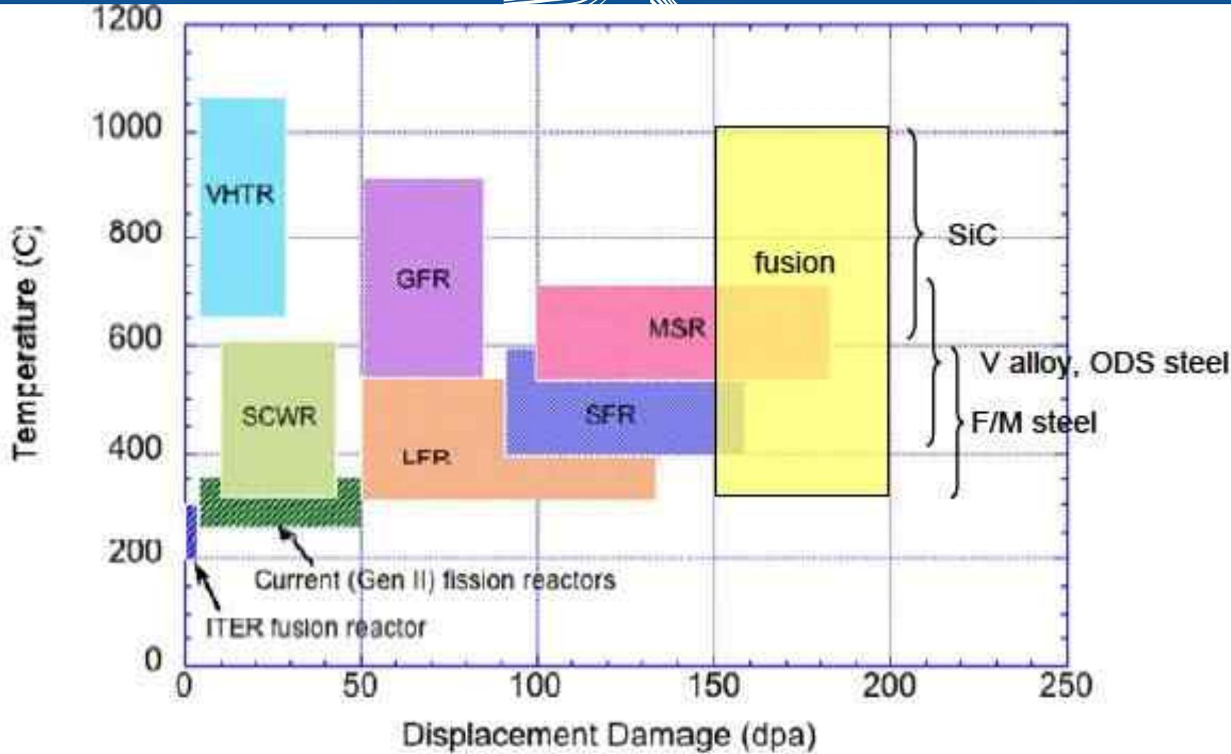
On top of thermal aging, fatigue and corrosion, irradiation damage is a key issue when considering extended reactor lifetimes. Since the materials within the reactor core could be used in an intense high-energy neutron field, it must exhibit good dimensional, mechanical and microstructural stability to neutron displacement damage. The radiation-resistance is often the most challenging requirement to evaluate since the key degradation mechanisms are sensitive to the specific radiation conditions.
