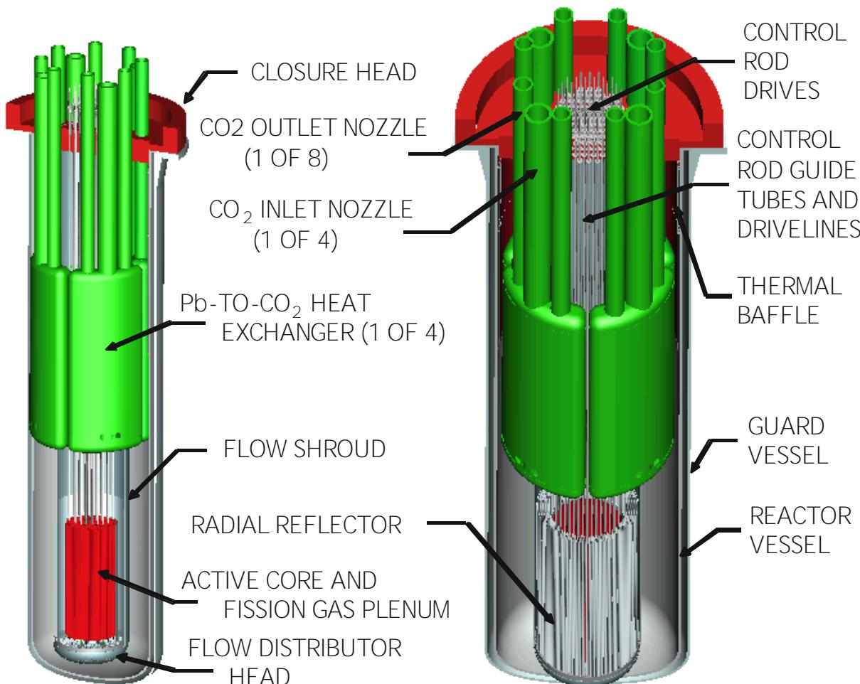
**SSTAR is a small natural circulation fast reactor of 20 MWe/45 MWt, that can be scaled up to 180 MWe/400 MWt.**
