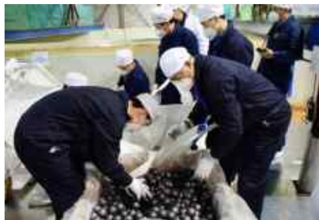
Workers inspect the spherical moderator elements prior to their loading
