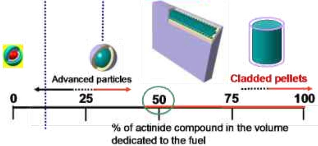
The greatest challenge facing GFR is the development of high temperature, high rating, high burn-up fuel that has good fission product retention and is tolerant to fault conditions.
