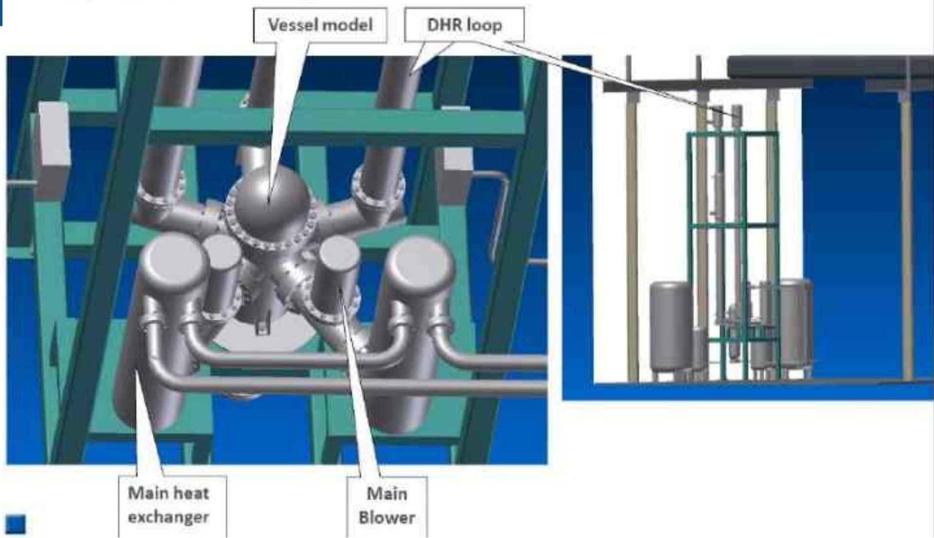
The experimental facility S-ALLEGRO (1 MW power) is located at Centrum výzkumu Řež s.r.o., Czech Republic. It is part of the EU Project “Sustainable Energy” (SUSEN) under Operation Programme “Research and Development for Innovations”. This facility will have two loops for normal operation with heat exchangers and circulators. There will be also three decay heat removal (DHR) loops.
