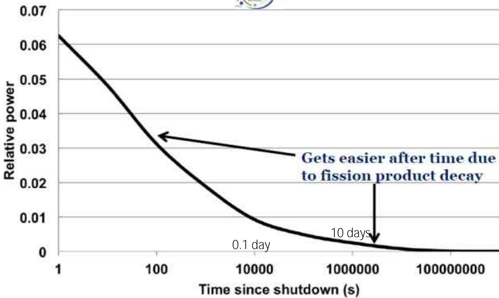
Relative power of 7 % = heat of about 200 MWth in the case of a 3000 MWth plant (i.e. 1 GWe reactor)
