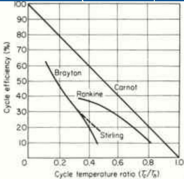
Figure left - Comparison of dynamic power conversion cycle typical efficiencies versus the temperature ratio between the cold and hot side of the cycle.
